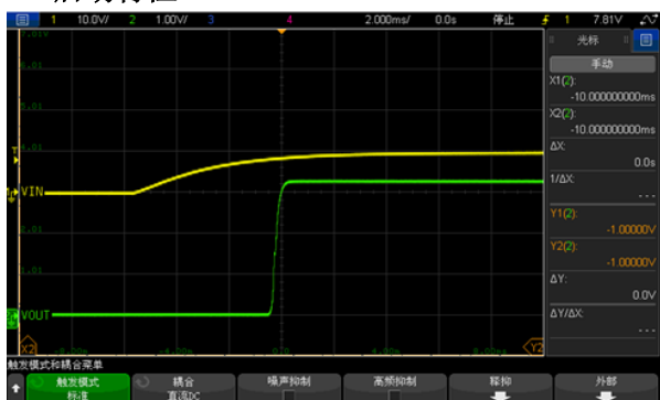
Vin=10V, Iout=0mA, Cout=0.1uF
