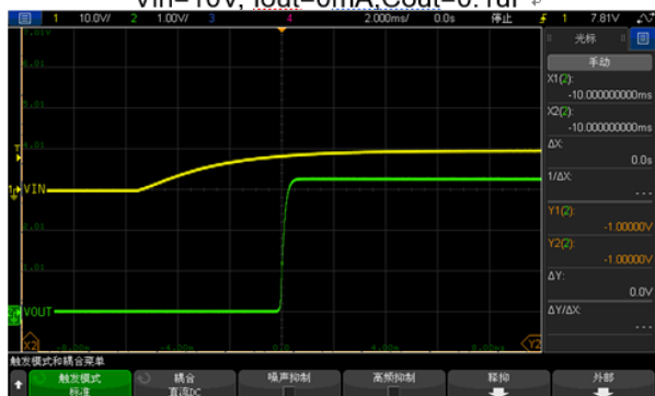
Vin=10V, Iout=30mA, Cout=0.1uF
